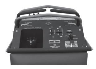
This photo shows the hydrostatic control levers are in the NEUTRAL position.
