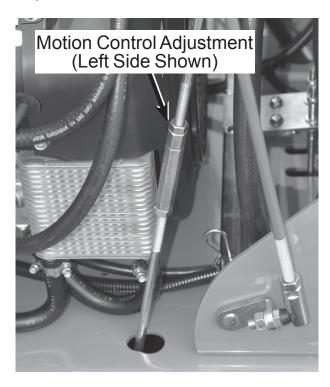
There are adjusters located by the transaxles on the control linkages. Loosen the jam nuts on the top and bottom of the adjuster.
