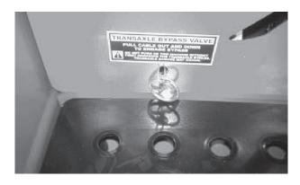
**Transaxle Bypass Valve Disengaged**
