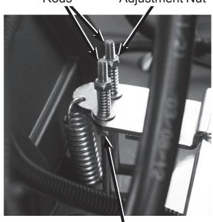
Brake Release Adjusting Nut
