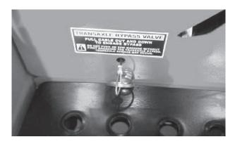
**Transaxle Bypass Valve Engaged**
