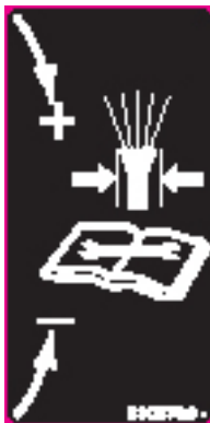
Figure 11: Spray Pressure Relief Valve Adjustment Decal (P/N 5105769)
